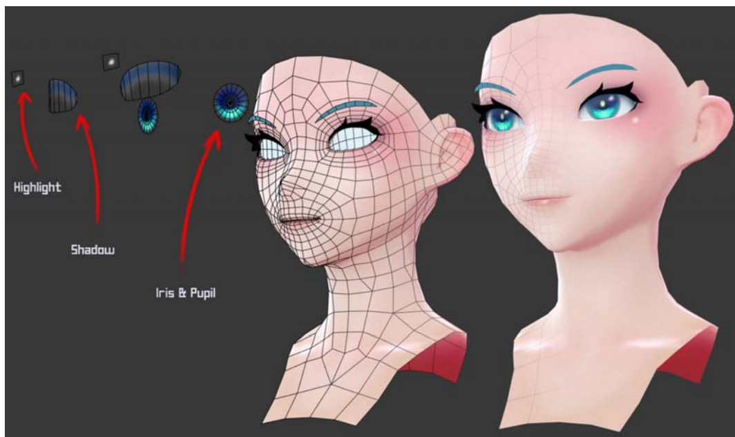
Figure 12 - 3D synthetic content created from a meshed 3D shape onto which 2D textures are added
