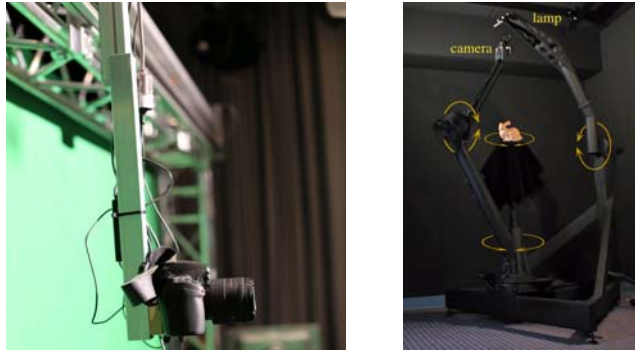
Figure 3 – Camera mounted on robot system (Fraunhofer IIS, Stanford [R3b])
