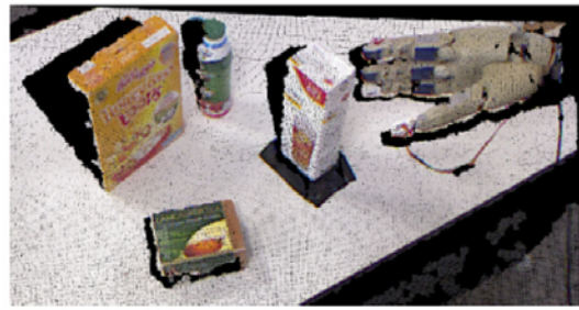
(b) 1 mm voxel resolution, 231618 points, 0.881 bpp , compression ratio 14
