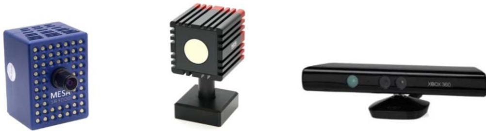
Figure 11 - Example depth cameras (from left to right): Mesa Imaging's Swiss Ranger SR3000 and SR4000, Microsoft Kinect 360.
