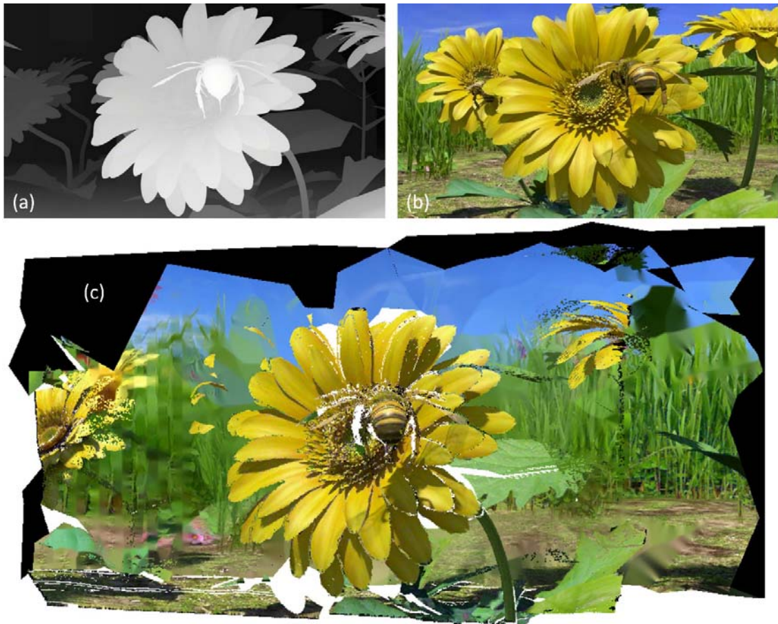
Figure 22 - Hybrid point cloud and piecewise planar representation (c) from depth maps (a) and projected views (b) [R22]
